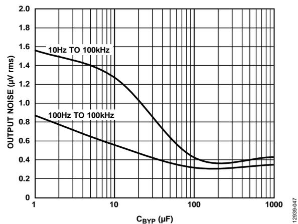
Figure 45. RMS Output Noise vs. Bypass Capacitance ( $C_{\text{BYP}}$ )
