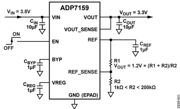
Figure 1. Regulated 3.3 V Output from 3.8 V Input
