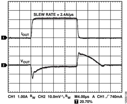
Figure 36. Load Transient Response,  $I_{LOAD} = 100\text{ mA}$  to  $2\text{ A}$ ,  $V_{OUT} = 1.8\text{ V}$ ,  $V_{IN} = 2.5\text{ V}$ ,  $C_{OUT} = 22\text{ }\mu\text{F}$ , Channel 1 =  $I_{OUT}$ , Channel 2 =  $V_{OUT}$
