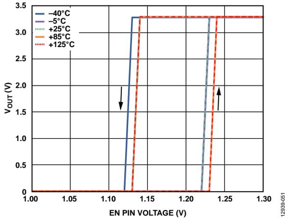
Figure 49. Typical V<sub>OUT</sub> Response to EN Pin Operation
