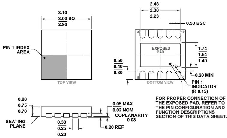
Figure 65. 10-Lead Lead Frame Chip Scale Package [LFCSPP]
