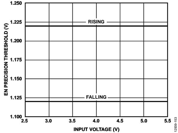
Figure 51. Typical EN Threshold vs. Input Voltage (V<sub>IN</sub>)
