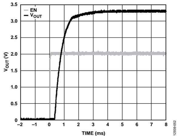
Figure 50. Typical V<sub>OUT</sub> Response to EN Pin Operation (V<sub>EN</sub>), V<sub>OUT</sub> = 3.3 V, V<sub>IN</sub> = 5 V, C<sub>BYP</sub> = 1 μF
