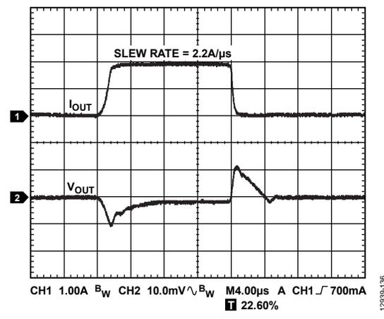
Figure 34. Load Transient Response,  $I_{LOAD} = 100\text{ mA}$  to  $2\text{ A}$ ,  $V_{OUT} = 3.3\text{ V}$ ,  $V_{IN} = 4.0\text{ V}$ ,  $C_{OUT} = 22\text{ }\mu\text{F}$ , Channel 1 =  $I_{OUT}$ , Channel 2 =  $V_{OUT}$
