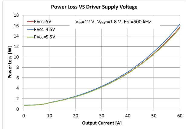
Figure 7. Power Loss vs. Driver Supply Voltage
