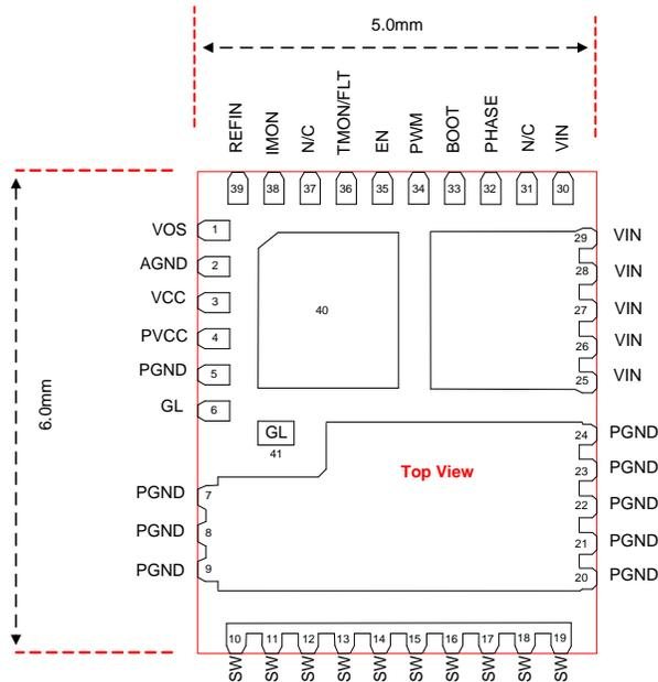
Figure 3. Pin Configuration
