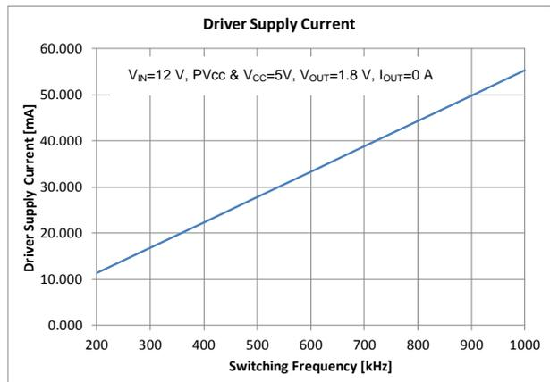
Figure 9. Driver Supply Current vs. Switching Frequency
