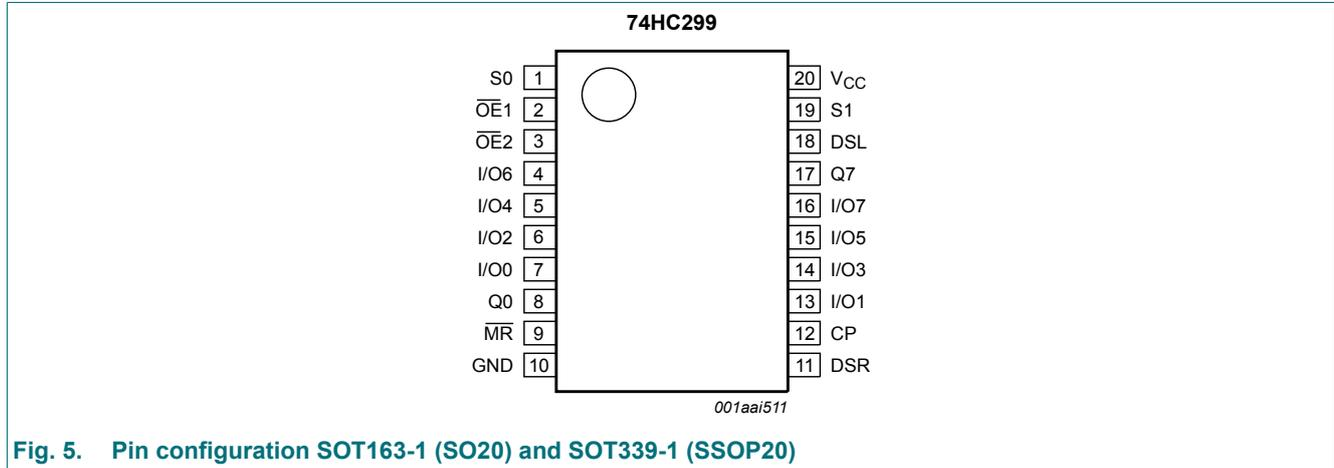
Fig. 5. Pin configuration SOT163-1 (SO20) and SOT339-1 (SSOP20)
