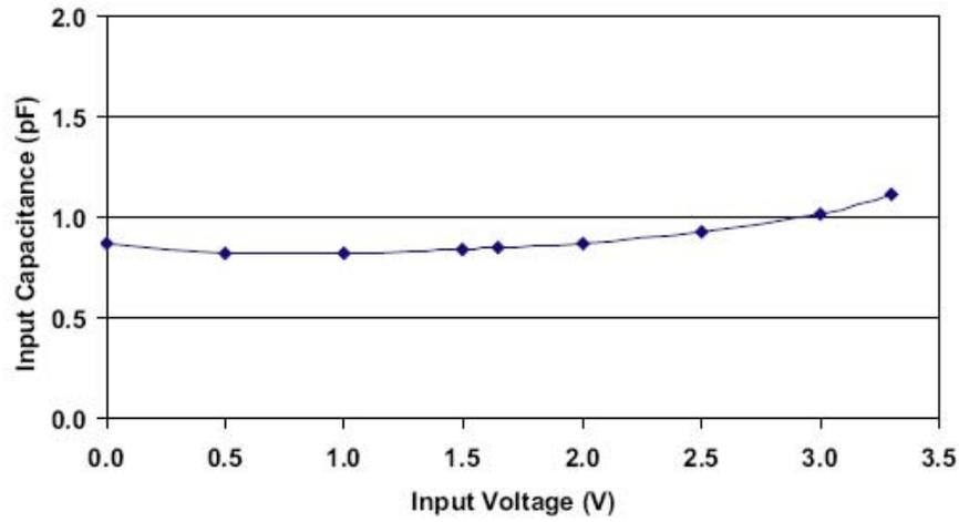
Figure 1. Typical Variation of  $C_{IN}$  vs.  $V_{IN}$
