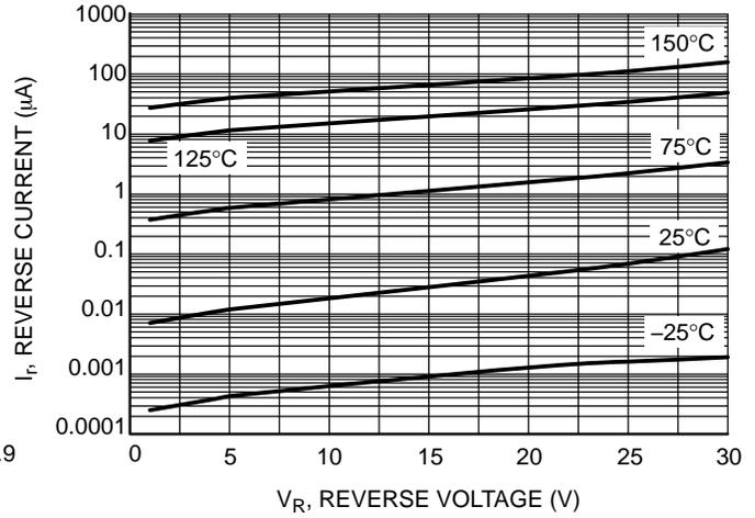
Figure 2. Leakage Current
