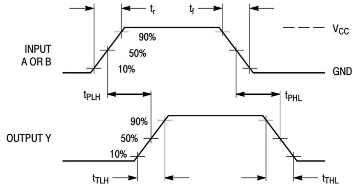
**Figure 1. Switching Waveforms**
