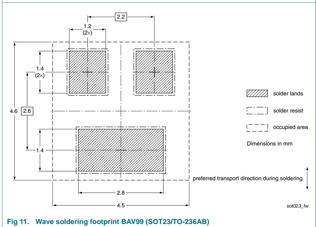
**Fig 11. Wave soldering footprint BAV99 (SOT23/TO-236AB)**
