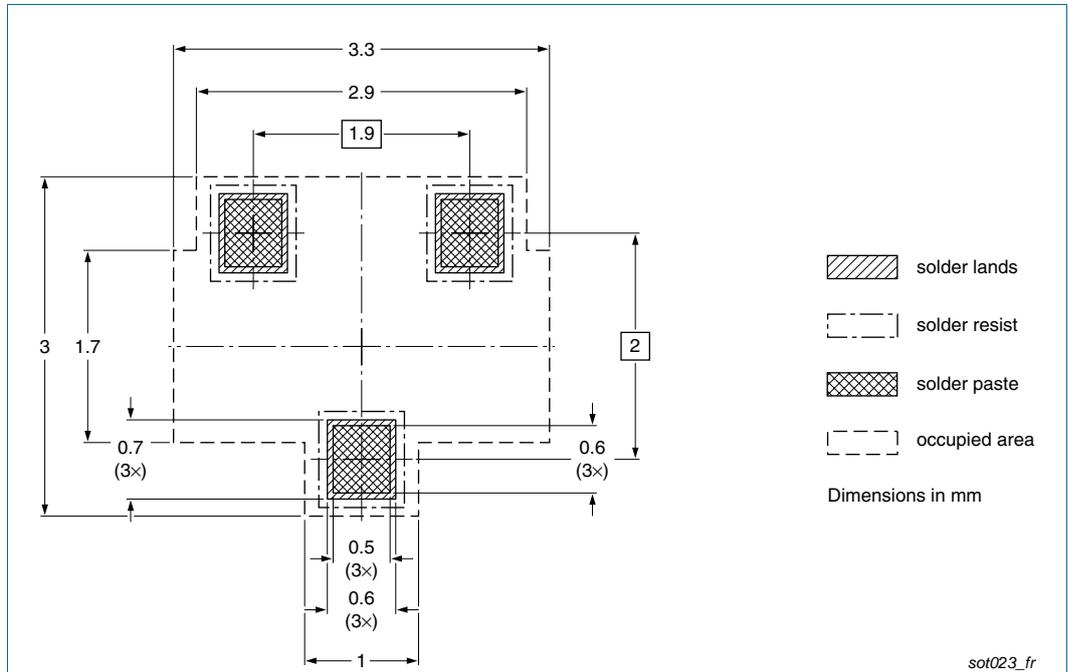
**Fig 10. Reflow soldering footprint BAV99 (SOT23/TO-236AB)**
