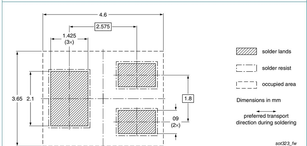
**Fig 15. Wave soldering footprint BAV99W (SOT323/SC-70)**
