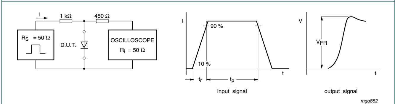
Input signal: forward pulse rise time  $t_r = 20 \text{ ns}$ ; forward current pulse duration  $t_p \geq 100 \text{ ns}$ ; duty cycle  $\delta \leq 0.005$
