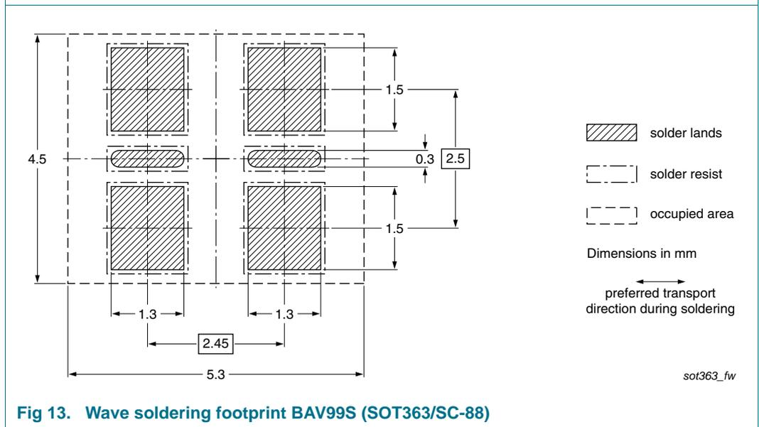
**Fig 13. Wave soldering footprint BAV99S (SOT363/SC-88)**
