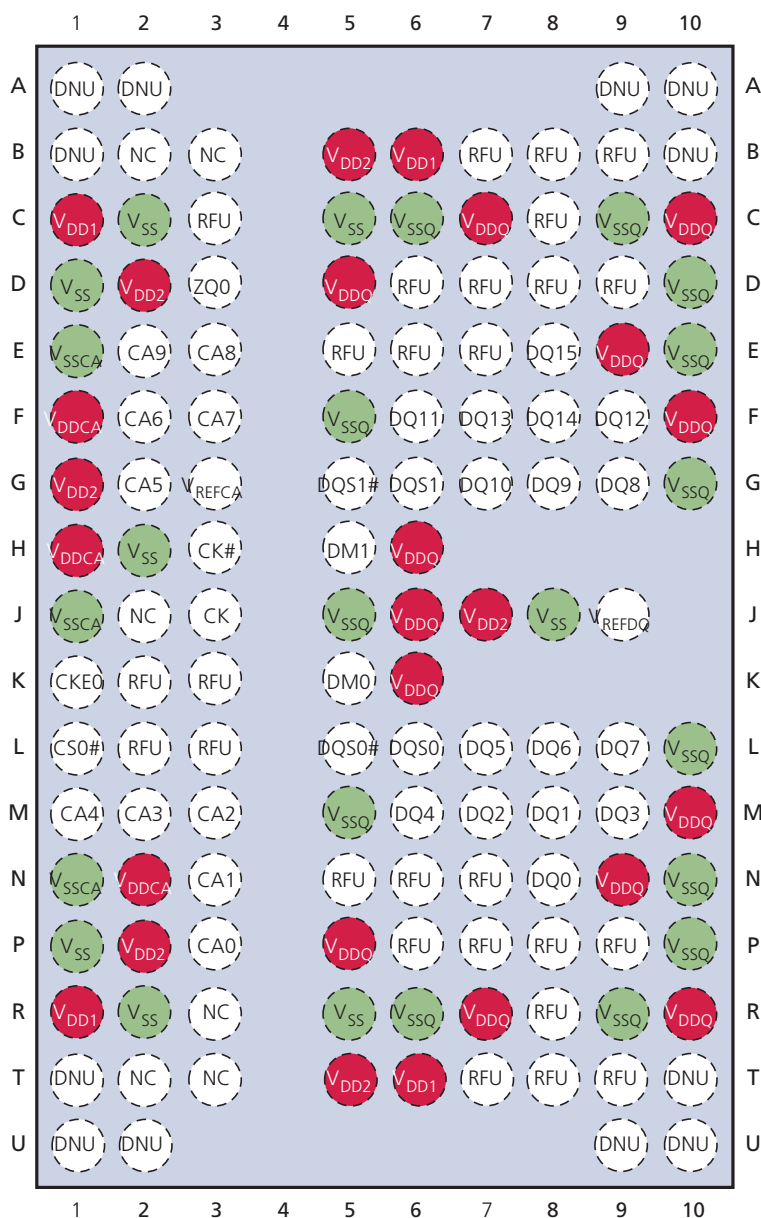
Figure 7: 134-Ball FBGA (64 Meg x16)
