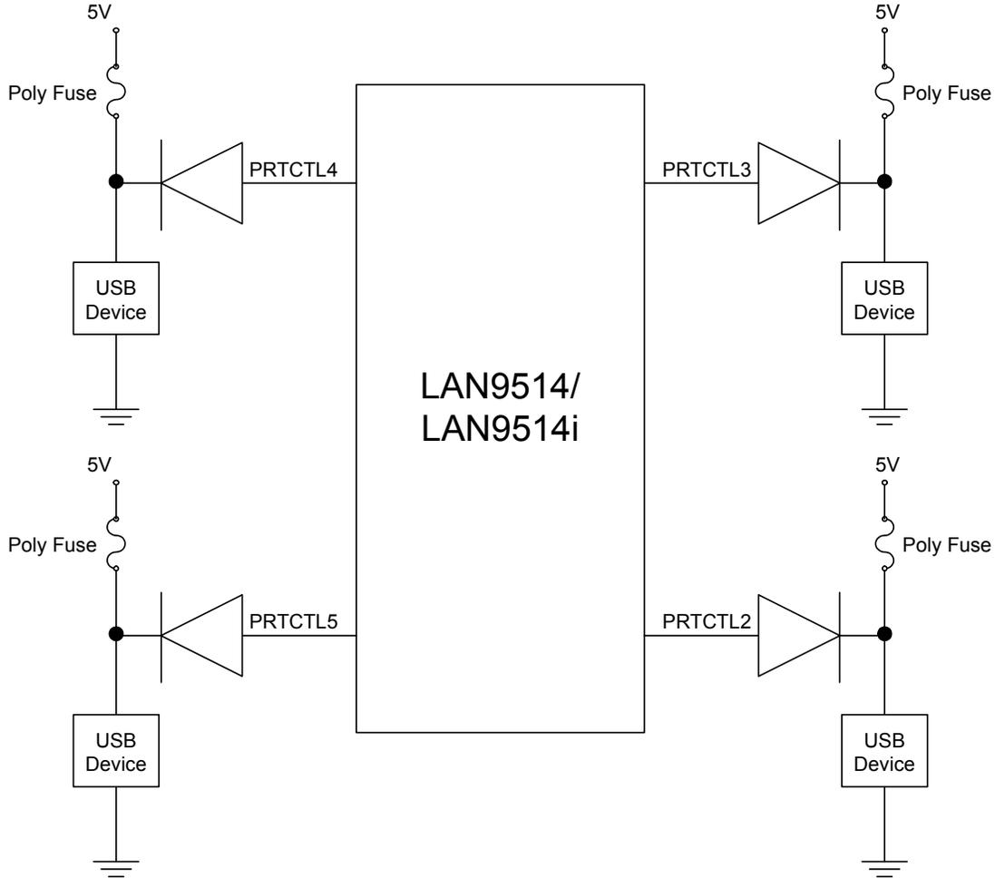
Many customers use a single poly fuse to power all their devices. For the ganged situation, all power control pins must be tied together.
