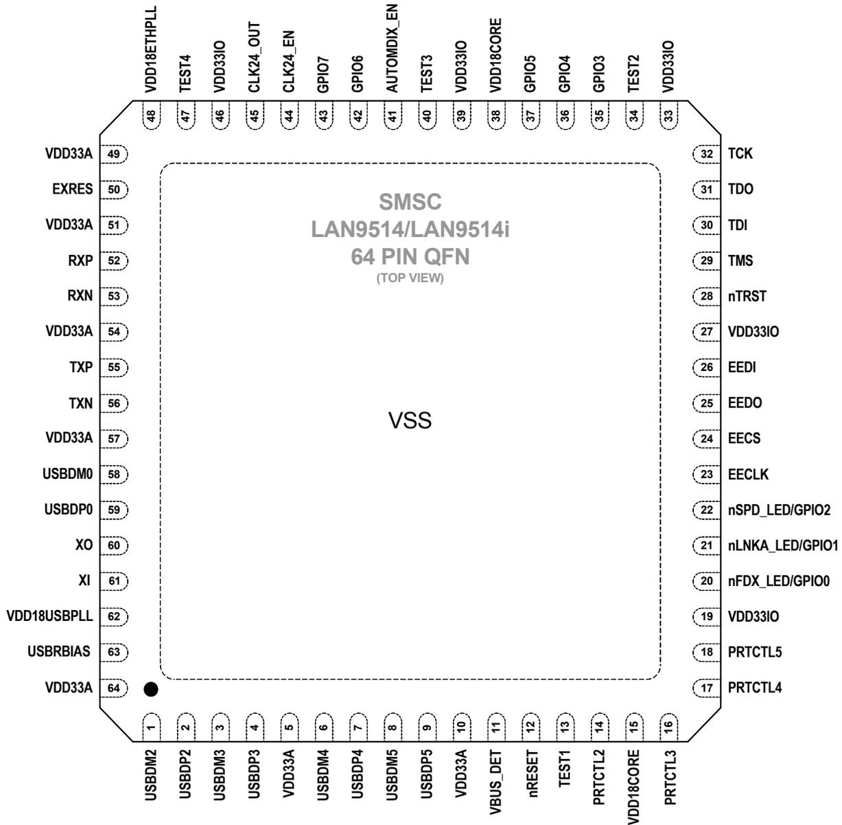
NOTE: When HP Auto-MDIX is activated, the TXN/TXP pins can function as RXN/RXP and vice-versa
