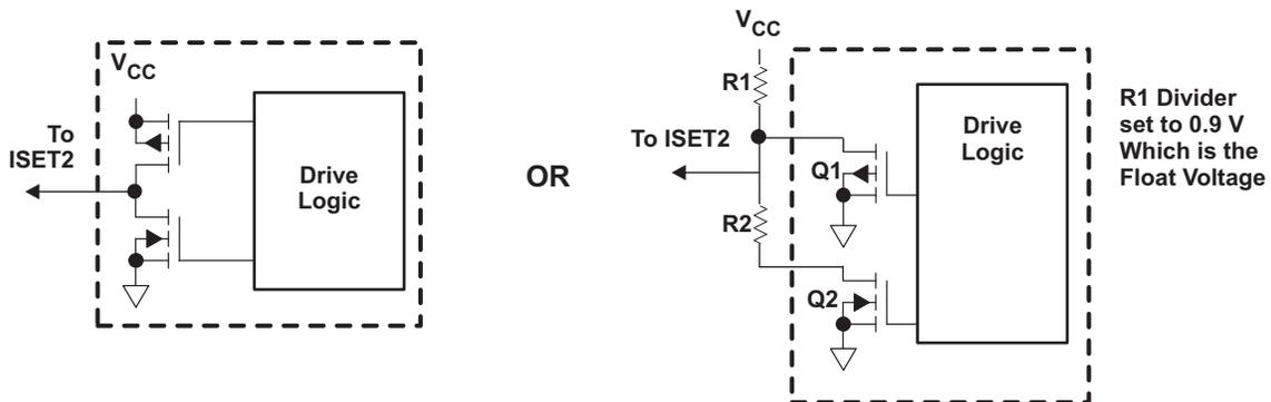
Figure 19. Configurations for Driving the 3-State ISET2 Pin
