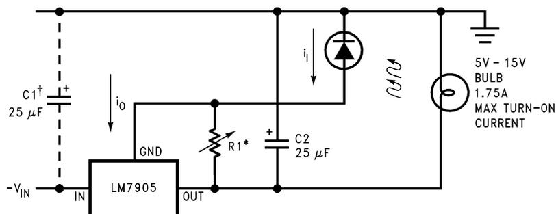
\*Lamp brightness increase until  $i_i = i_Q (\approx 1 \text{ mA}) + 5\text{V}/R1$ .
