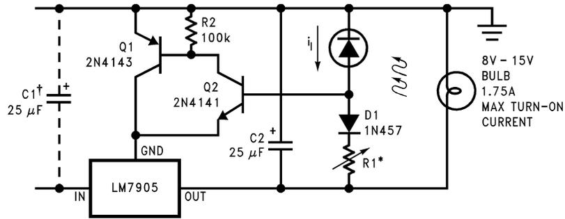
\*Lamp brightness increases until  $i_i = 5V/R1$  ( $i_i$  can be set as low as  $1 \mu A$ )
