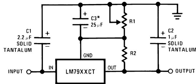
\*Improves transient response and ripple rejection. Do not increase beyond  $50 \mu F$ .
