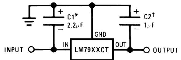
\*Required if regulator is separated from filter capacitor by more than 3". For value given, capacitor must be solid tantalum. 25µF aluminum electrolytic may be substituted.
