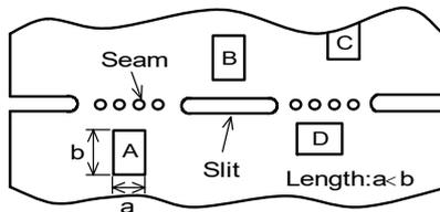
\*1 A > D is valid when stress is added vertically to the perforation as with Hand Separation. If a Cutting Disc is used, stress will be diagonal to the PCB, therefore A > D is invalid.
