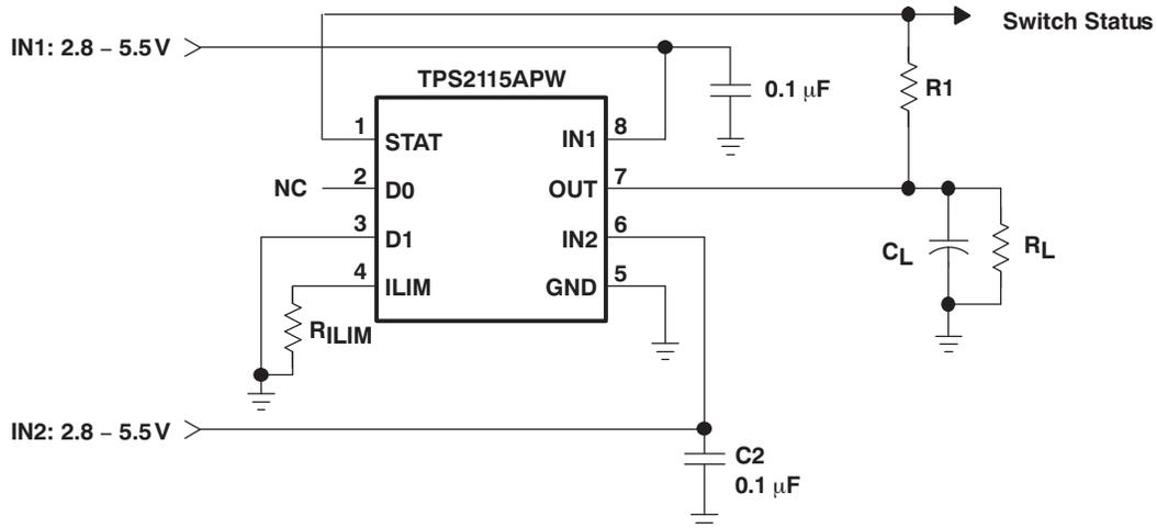
Figure 14. Auto-Selecting for a Dual Power Supply Application
