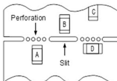
(3) Mounting components near screw holes
