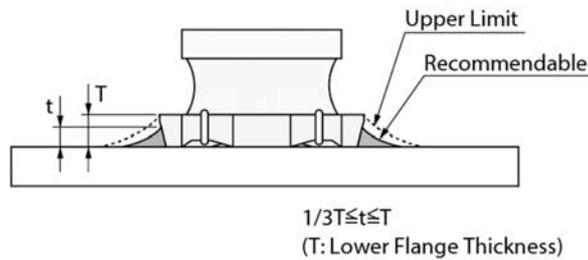
An increased solder volume increases mechanical stress on the product. Exceeding solder volume may cause the failure of mechanical or electrical performance.
