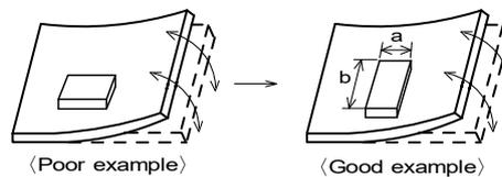
(2) Components location on PCB separation
