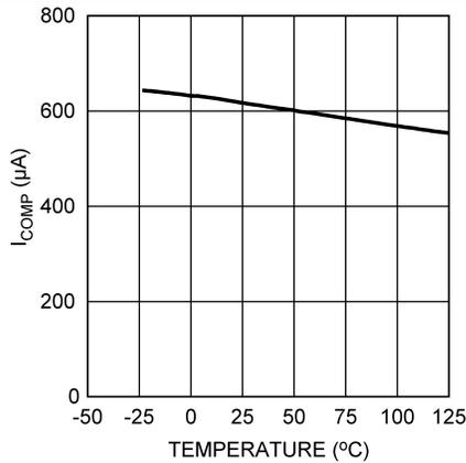
Figure 9. COMP Pin Source Current vs. Temperature
