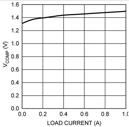
**Figure 3. Comp Pin Voltage vs. Load Current**
