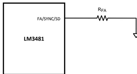
**Figure 25. Frequency Adjust**
