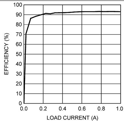
**Figure 6. Efficiency vs. Load Current (5  $V_{IN}$  and 12  $V_{OUT}$ )**
