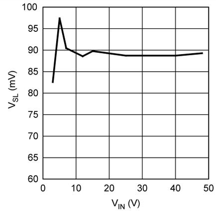
**Figure 16. Compensation Ramp Amplitude vs. Input Voltage**
