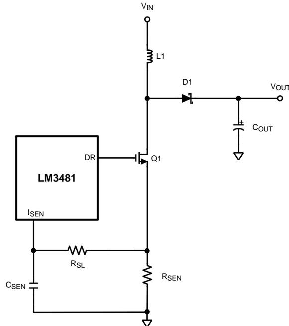
Figure 23. Increasing the Slope of the Compensation Ramp
