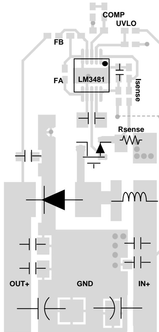
Figure 39. Typical Layout for a Boost Converter
