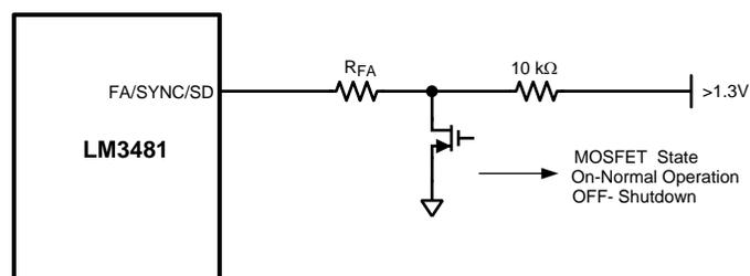
**Figure 27. Shutdown Operation in Frequency Adjust Mode**
