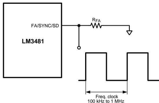
**Figure 26. Frequency Synchronization**
