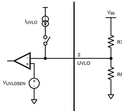
Figure 29. UVLO Pin Resistor Divider
