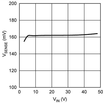
**Figure 15. Current Sense Threshold vs. Input Voltage**
