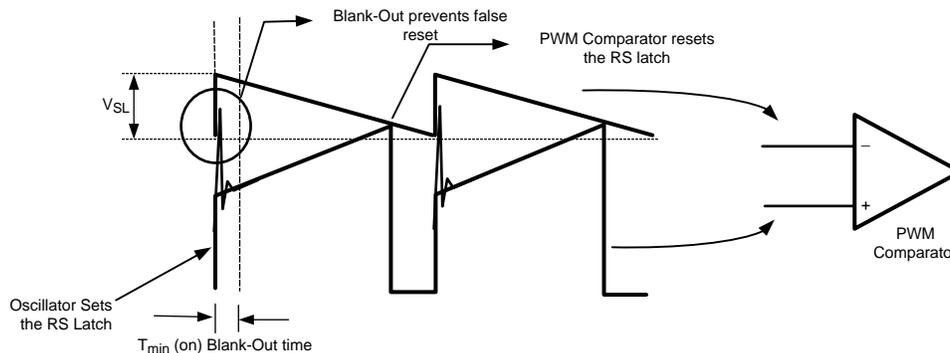
Figure 18. Basic Operation of the PWM Comparator
