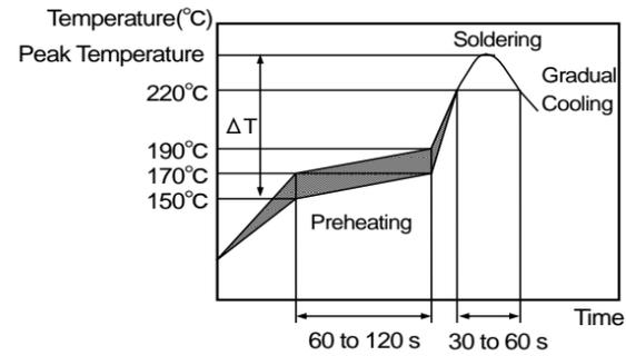
[Allowable Reflow Soldering Temperature and Time]
