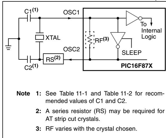
**FIGURE 11-2: EXTERNAL CLOCK INPUT OPERATION (HS, XT OR LP OSC CONFIGURATION)**
