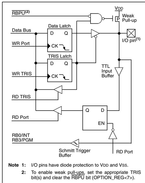
Four of the PORTB pins, RB7:RB4, have an interrupt-on-change feature. Only pins configured as inputs can cause this interrupt to occur (i.e., any RB7:RB4 pin configured as an output is excluded from the interrupt-on-change comparison). The input pins (of RB7:RB4) are compared with the old value latched on the last read of PORTB. The "mismatch" outputs of RB7:RB4 are OR'ed together to generate the RB Port Change Interrupt with flag bit RBIF (INTCON<0>).
