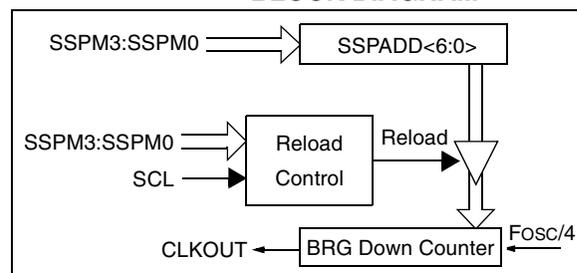
**FIGURE 9-11: BAUD RATE GENERATOR TIMING WITH CLOCK ARBITRATION**
