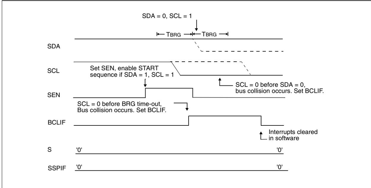
**FIGURE 9-22: BRG RESET DUE TO SDA COLLISION DURING START CONDITION**
