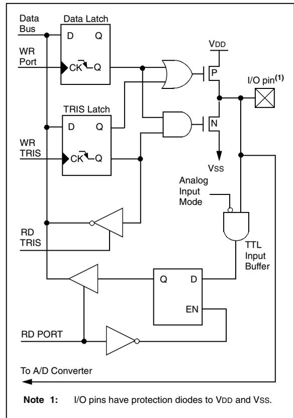
**FIGURE 4-2: BLOCK DIAGRAM OF RA4/T0CKI PIN**
