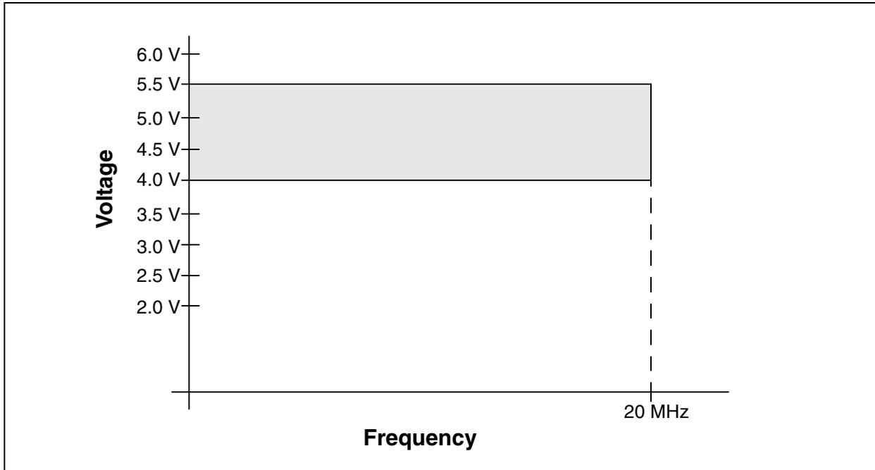
FIGURE 14-2: PIC16LF872 VOLTAGE-FREQUENCY GRAPH
