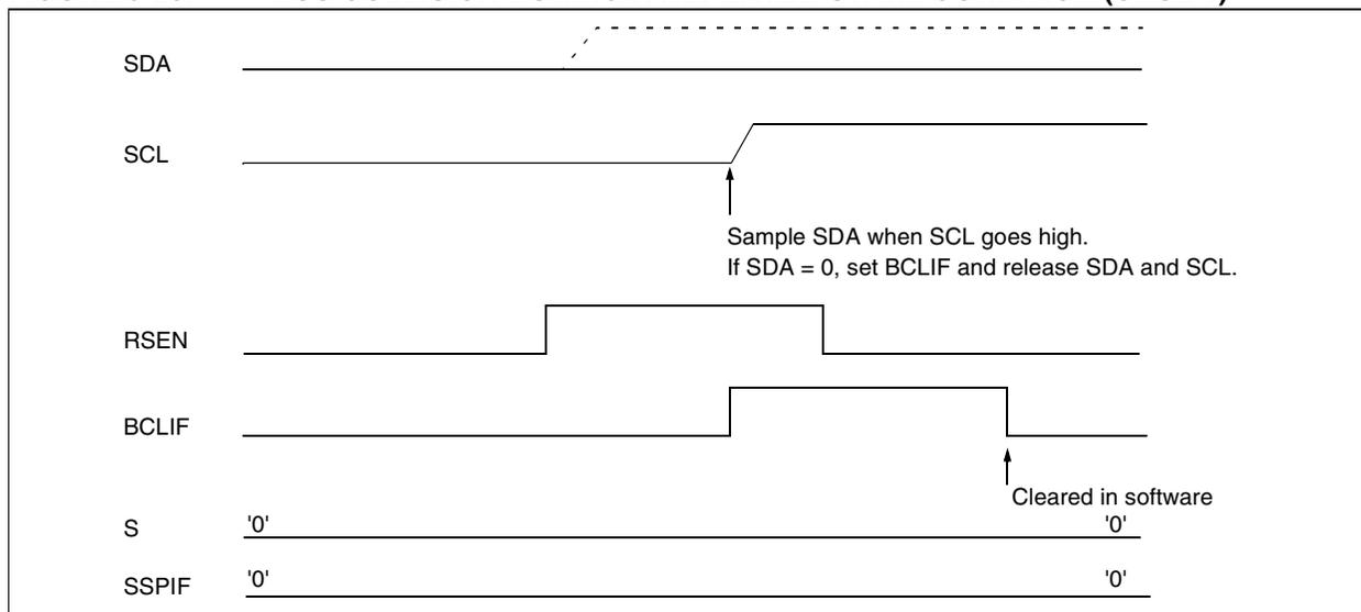
**FIGURE 9-24: BUS COLLISION DURING REPEATED START CONDITION (CASE 2)**
