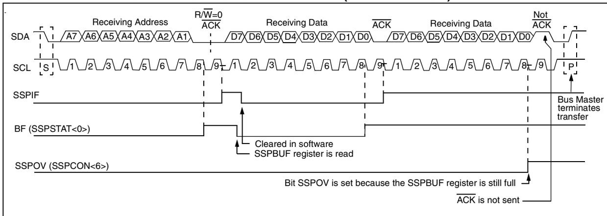
**FIGURE 9-7: I<sup>2</sup>C WAVEFORMS FOR TRANSMISSION (7-BIT ADDRESS)**
