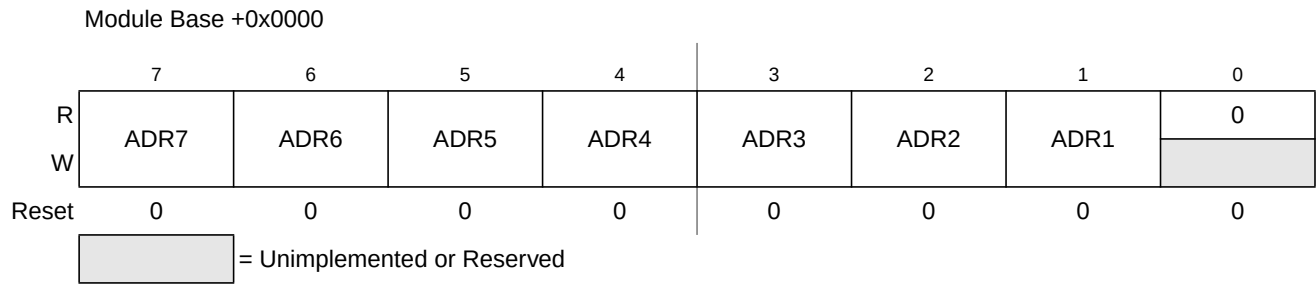
Figure 10-3. IIC Bus Address Register (IBAD)
