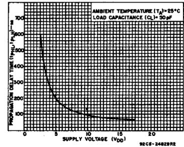
Fig. 10 - Typical propagation delay time vs. supply voltage.
