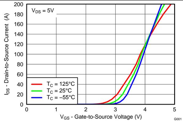
Figure 3. Transfer Characteristics
