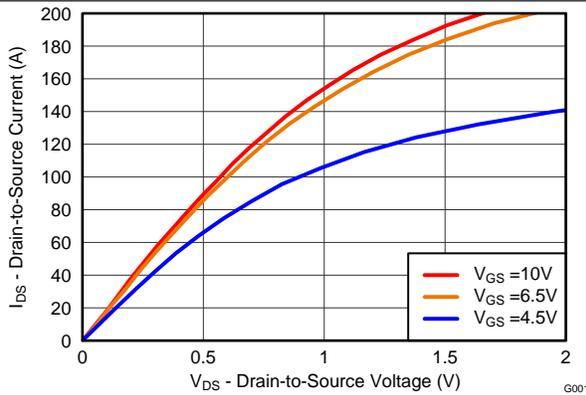
Figure 2. Saturation Characteristics
