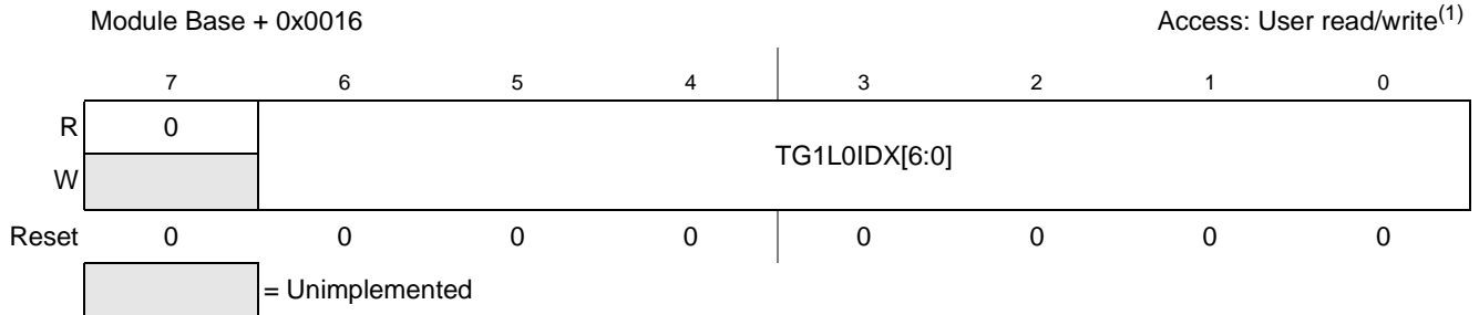
Figure 13-19. Trigger Generator 1 List 0 Index (TG1L0IDX)
