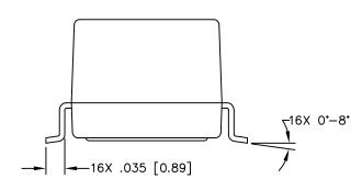
DIMENSIONS ARE IN INCHES [MILLIMETERS] WITH THE FOLLOWING TOLERANCES: [MILLIMETERS] ARE FOR REFERENCE ONLY. .XX=  $\pm$ .01 [ $\pm$ 0.25] .XXX=  $\pm$ .005 [ $\pm$ 0.13]
